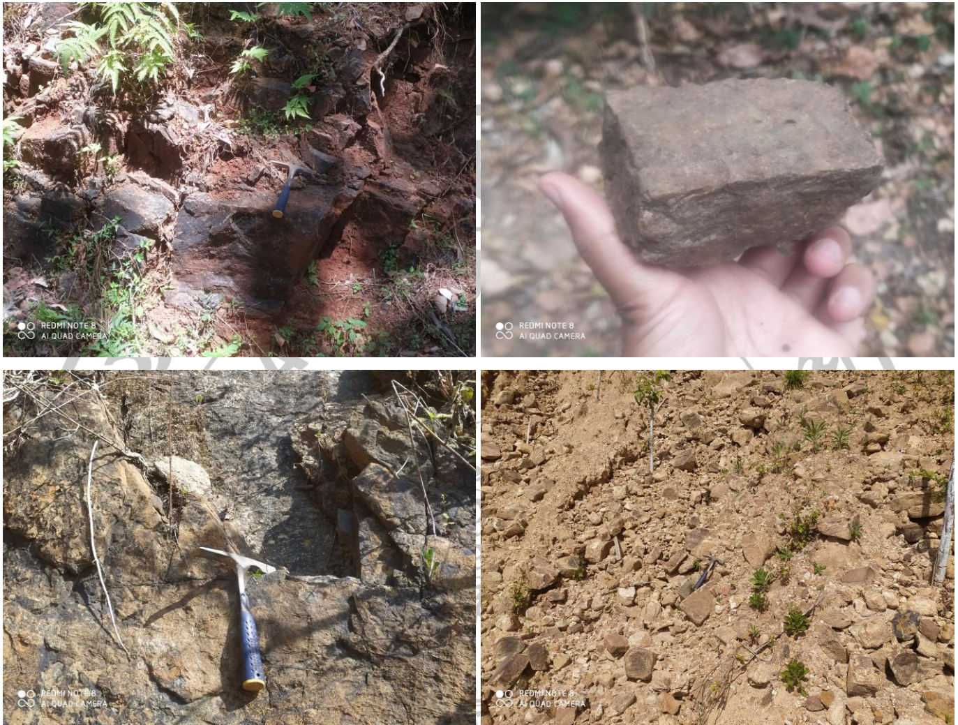
Figure-2.6: Disintegration of rock into smaller orthogonal pieces due to joint interference impact in the study area
